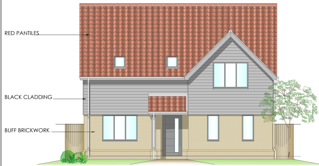
Front (North West) Elevation
