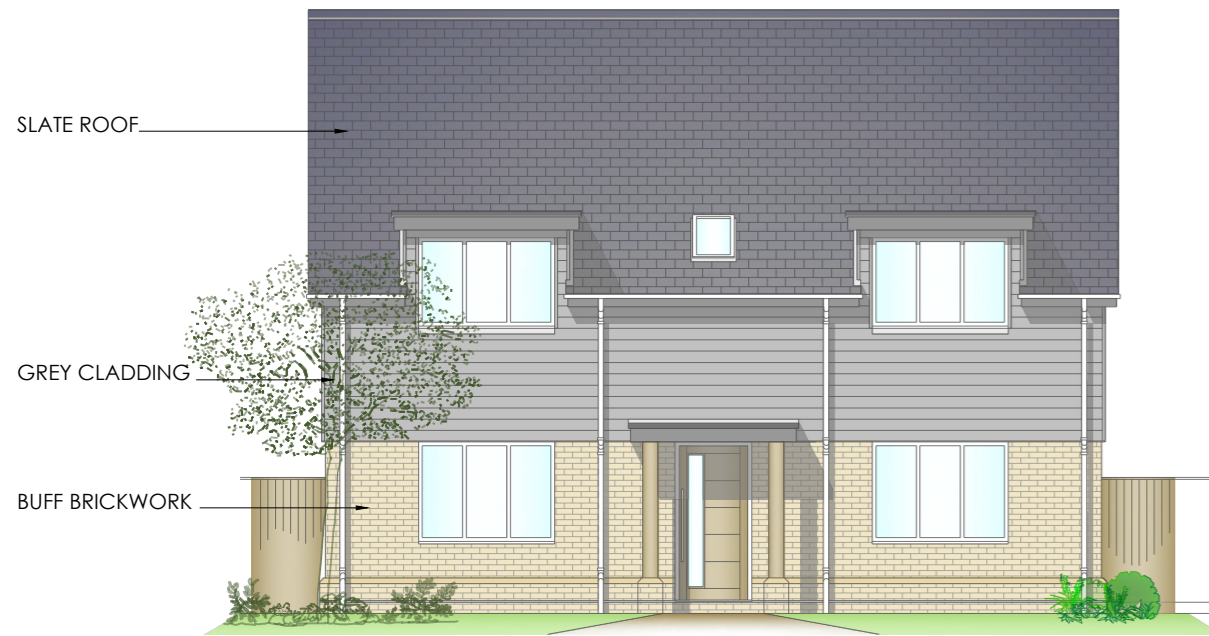
Front (South East) Elevation
